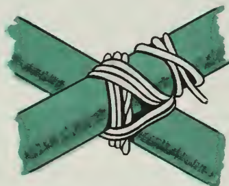
Diagonal lashing completed
