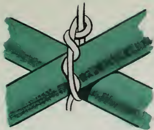
Timber hitch loose
