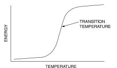
Impact tests determine the amount of energy required to cause
