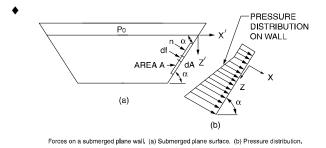
The pressure on a point at a distance Z' below the surface is
