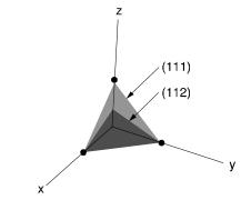
(111) plane. (axis intercepts at x = y = z) (112) plane. (axis intercepts at x = 1, y = 1, z = 1/2)
