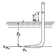
For a *compressible fluid*, use the above incompressible fluid equation if the mach number  $\leq 0.3$ .
