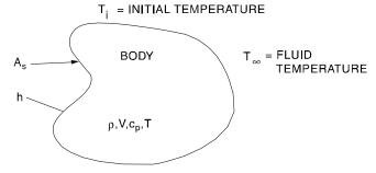
If the temperature may be considered uniform within the body at any time, the change of body temperature is given by
