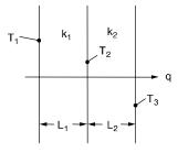
$R_{\text{total}} = R_1 + R_2$ , where
