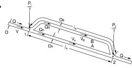
The same head loss occurs in each branch as in the combination of the two. The following equations may be solved simultaneously for  $V_A$  and  $V_B$ :
