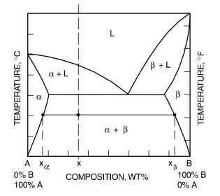
(In diagram, L = liquid) If x = the average composition at temperature T, then
