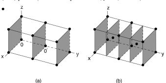
(010) planes in cubic structures. (*a*) Simple cubic. (*b*) BCC. (axis intercepts at  $x = \infty$ , y = 1,  $z = \infty$ )
