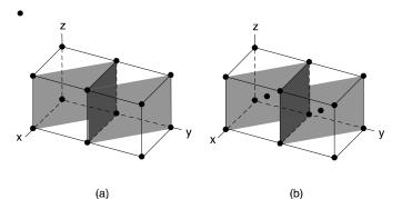
(110) planes in cubic structures. (a) Simple cubic. (b) BCC. (axis intercepts at  $x = 1, y = 1, z = \infty$ )
