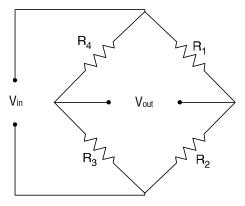
Half-bridge and full-bridge configurations use two or four variable resistors, respectively. A full-bridge strain gage circuit give a voltage output of
