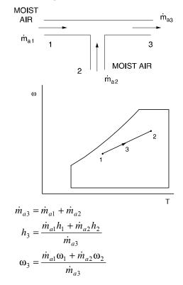
distance  $\overline{13} = \frac{\dot{m}_{a2}}{\dot{m}_{a3}}$  × distance  $\overline{12}$  measured on psychrometric chart
