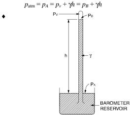
$p_v$  = vapor pressure of the barometer fluid
