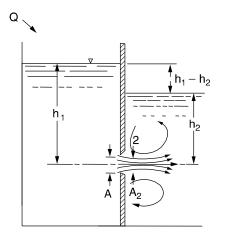
$$Q = A_2 V_2 = C_c C_v A \sqrt{2g(h_1 - h_2)}$$
