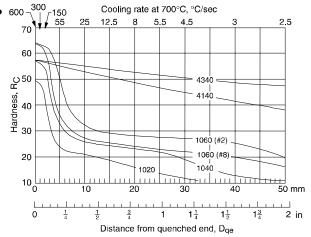
(#2) and (#8) indicated ASTM grain size
