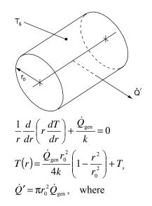
$\dot{Q}'$  = the heat-transfer rate from the cylinder per unit length.
