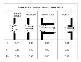
Submerged Orifice operating under steady-flow conditions:
