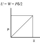
The strain energy per unit volume is  $u = U/AL = \sigma^2/2E$
