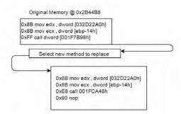
Changing a relative call is fairly easy as you just overwrite the 4 bytes of the immediate with the new destination address. Gray Storm has the ability to use an arbitrary address in a call instruction thanks to Reflection.
