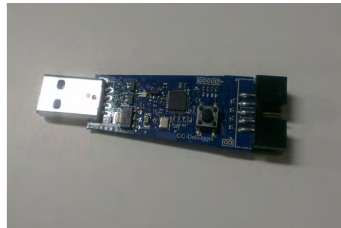
Debugger used to extract firmware
